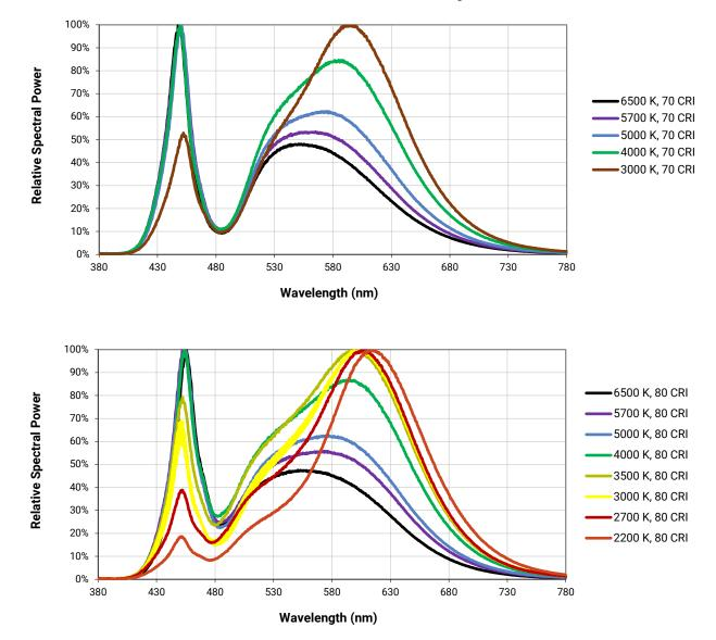
The following graphs are the result of a series of pulsed measurements at 1400 mA and T<sub>1</sub> = 85 °C.
